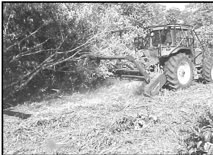
Figura 6 – Máquina utilizada para corte e trituração da biomassa vegetal (fresador florestal modelo AHWI-600). Fonte: FREITAS, A.C.R. Evaluating Agricultural Systems Based on Mulch Technology: A Case Study. International Research on Food Security, Natural Resource Management and Rural Development, 2005.
