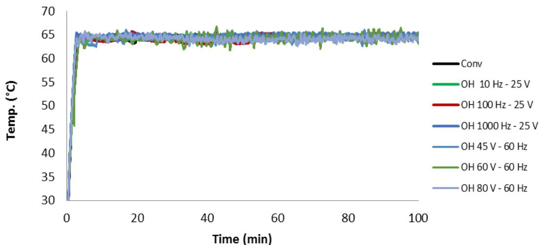
**Fig. 1.** Temperature profiles of conventional processing and Ohmic heating
