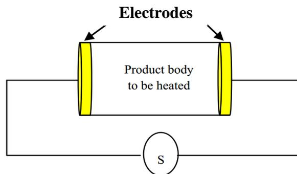
**Fig 1.** Basic Scheme of Ohmic Heating
