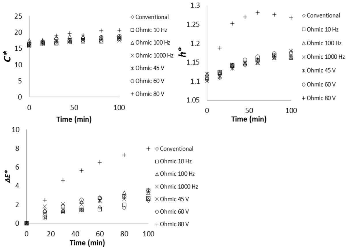
**Fig. 3.** Color parameters of whey-acerola flavored drink during Ohmic Heating and conventional processing
