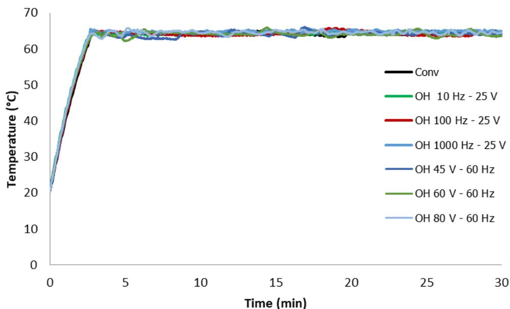
**Fig. 2.** Temperature profiles of Whey acerola-flavoured drink submitted to conventional processing and Ohmic Heating
