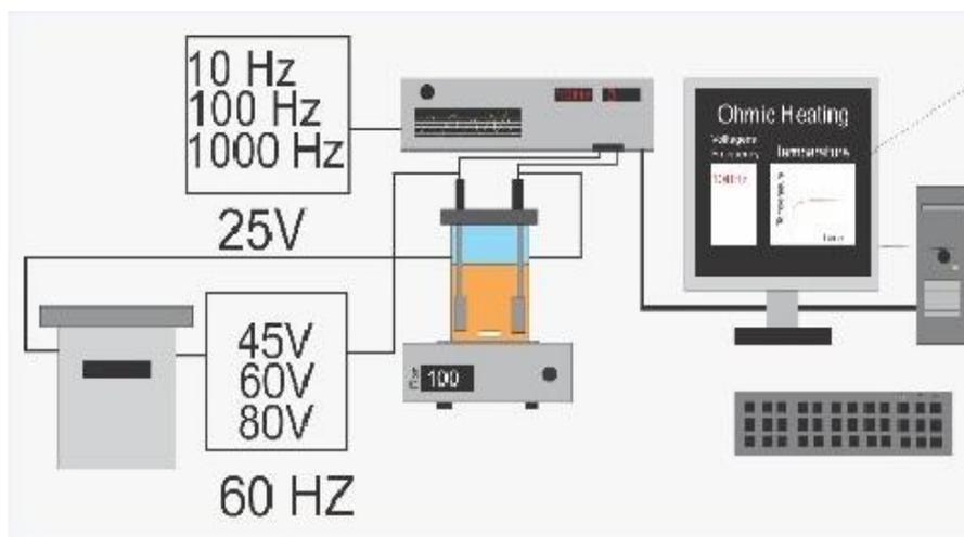
**Fig. 1.** Schematic diagram of the OH setup.
